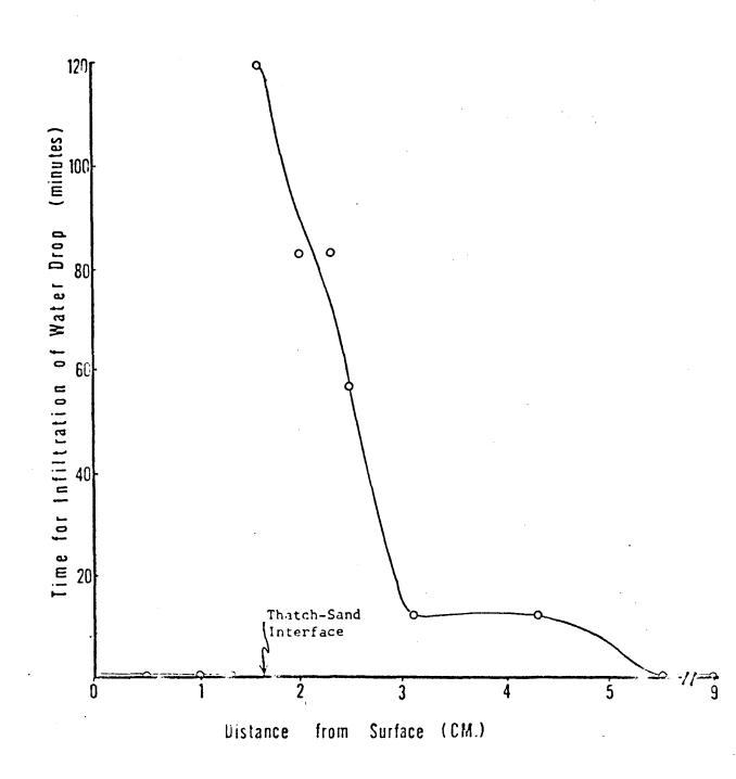
since the moist thatch readily absorbed water while the sand directly below was still dry. As soon as the water reached the nonwettable sand surface in the field it moved horizontally until it reached an area of wettable sand and moved down into the sand.
