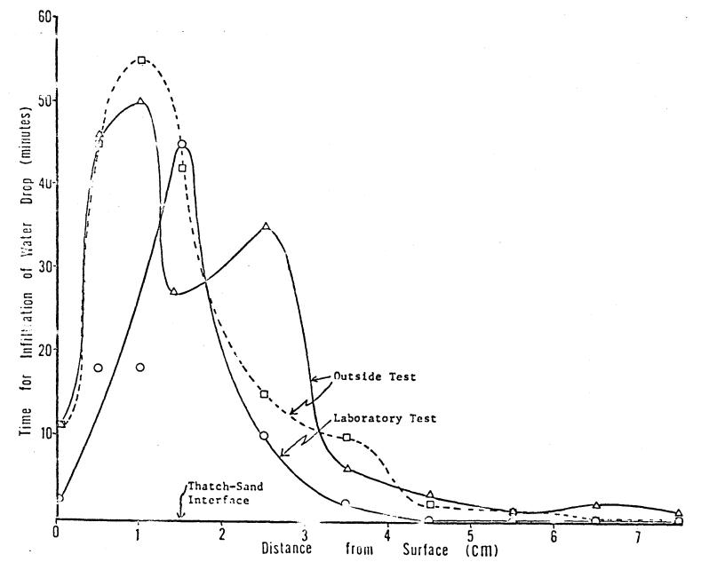
Figure 9. Absorption time of a wettable core (from experimental green) after drying at room temperature. Note the difference between this core and those that underwent slow drying in the water baths while enclosed in test tubes. (Figures 6, 7, 8).
