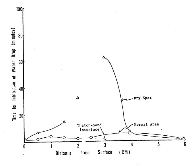
Figure 3. Average infiltration time of twelve nonwettable cores from the U.C. Experimental Green. The standard deviation for the 1-5 cm values was 30 minutes.
