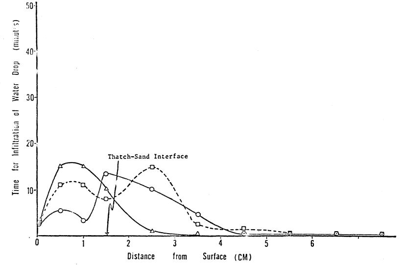
Figure 7. Absorption times of cores from slow drying experiment in direct sunlight. Two cores were dried outside in a 20°C water bath. Cores were tested immediately upon removal om water bath.
