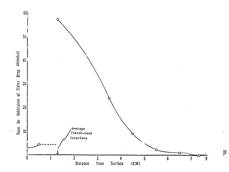
Figure 4. Example of infiltration time of a dry spot core from the experimental green, U.C. Davis, showing the dramatic increase in infiltration time at the thatch-sand interface, even when the core has been dried at room temperature.
