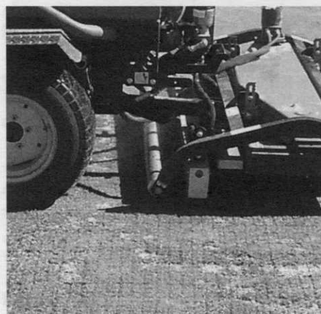
Figure 4. Side view of Envirojet inserting seed into weak and damaged turf.
