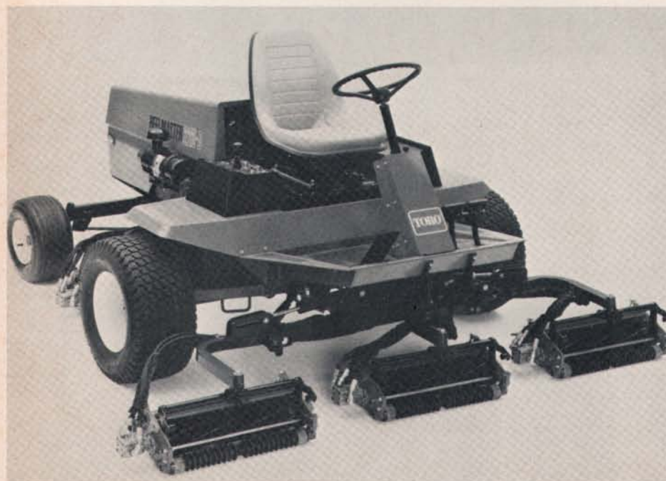
Toro Reelmaster 223-D lightweight fairway mower.
