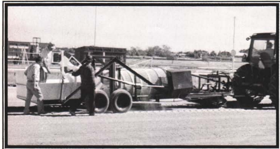
Rocks and debris are periodically removed from the dirt course with a rockpicker.
