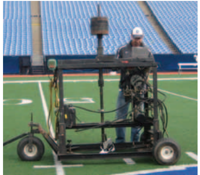
Figure 2. We test traction using Pennfoot - a device that allows us to compare traction levels on playing surfaces using various types of shoes.
