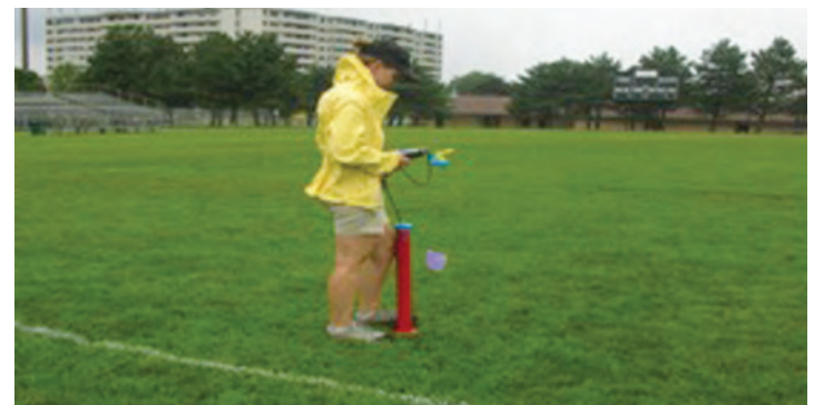
Figure 3. Clegg hammer impact tester used to determine surface hardness
