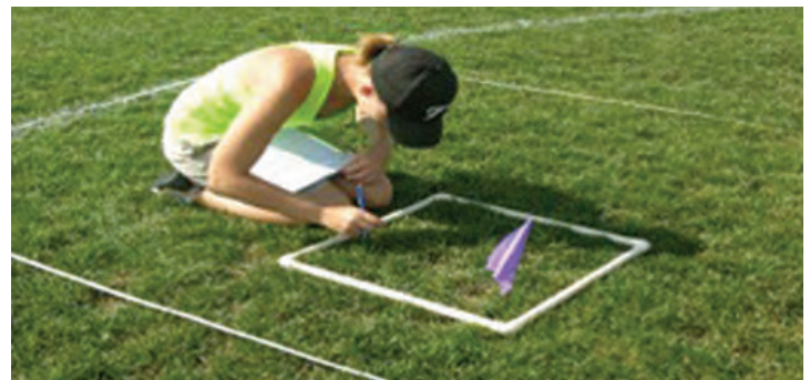
Figure 2. Point quadrat used to measure percent cover
