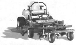
The JRCO aerator fits commercial walk behind and riding mowers. The 38-inch-wide unit can aerate 66,000 square feet per hour at 5 mph. Aeration holes are up to 3 inches deep, and the unit dispenses loose plugs of soil, not hard core plugs. There is no subsurface compaction around or at the bottom of the holes, which promotes water and air filtration. Video available showing this and other mower attachments.
