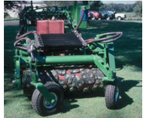
Dr. Bill Meyer has created a traffic machine with spikeless golf shoe soles for screening cool-season grasses at Rutgers University.
