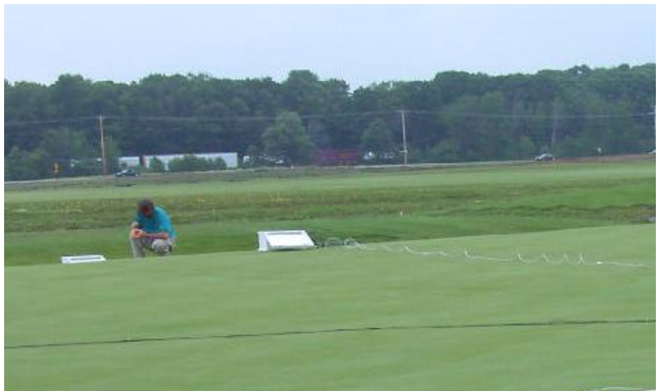
At Michigan State University, sloping greens with constant or variable sand rootzone mixtures were developed to study water movement through bentgrass putting greens.
