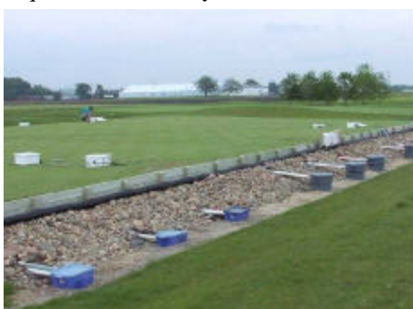
By altering the rootzone depth decreased soil moisture content at the 0-4 inch depth in low areas of the green and increased soil moisture content in high areas of the green.
