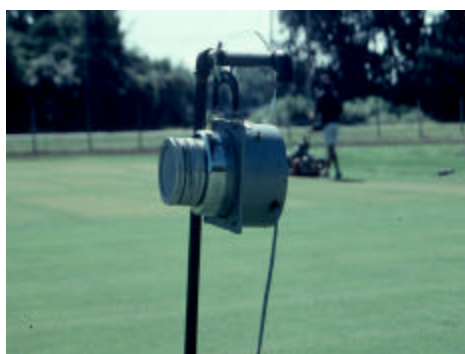
A high speed air sampler was used to measure the volatilization of several pesticides. This information has been translated into a model that accurately predicts pesticide volatilization under a range of environmental conditions.
