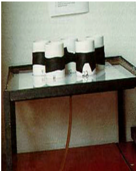
The rootzone test methods to determine saturated hydraulic conductivity are being evaluated in order to improve accuracy and precision.
