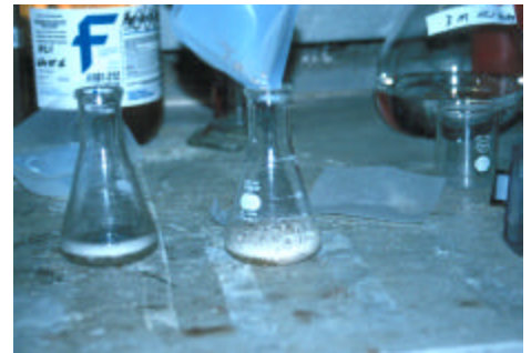
Acid added to calcareous sand demonstrates potential chemical instability.
