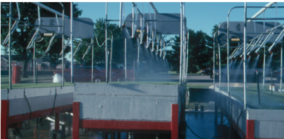
Rainfall simulators were used to evaluate the soil hydrology of two putting green rootzones at three different slopes in Phase I.
