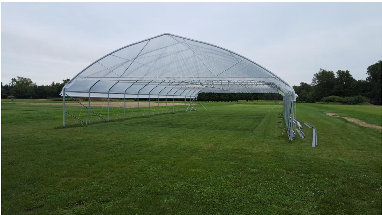
Figure 2. Rain-exclusion shelters are used to simulate 100-day drought periods in higher rainfall regions.
