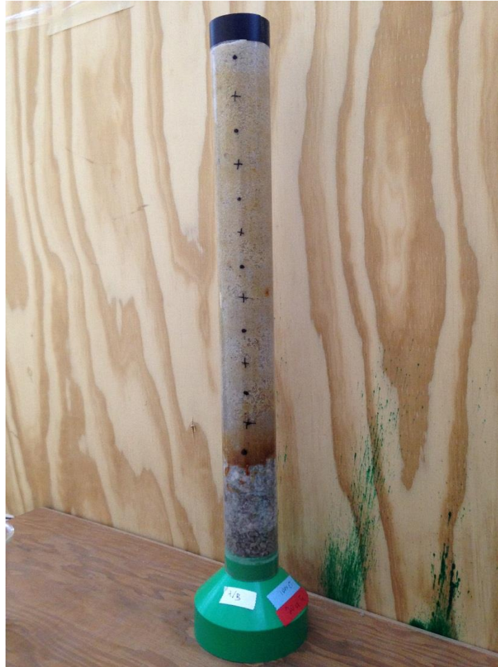
Figure 3. Iron-cemented layer at the sand/gravel interface of a root zone with a low-pH sand and a high-pH gravel. The column received eight total applications of Fe at a rate of 200 \text{ kg FeSO}_4 \text{ ha}^{-1} . Despite the visual observation of iron accumulation, there was no measured decrease in air infiltration rate after eight applications.
