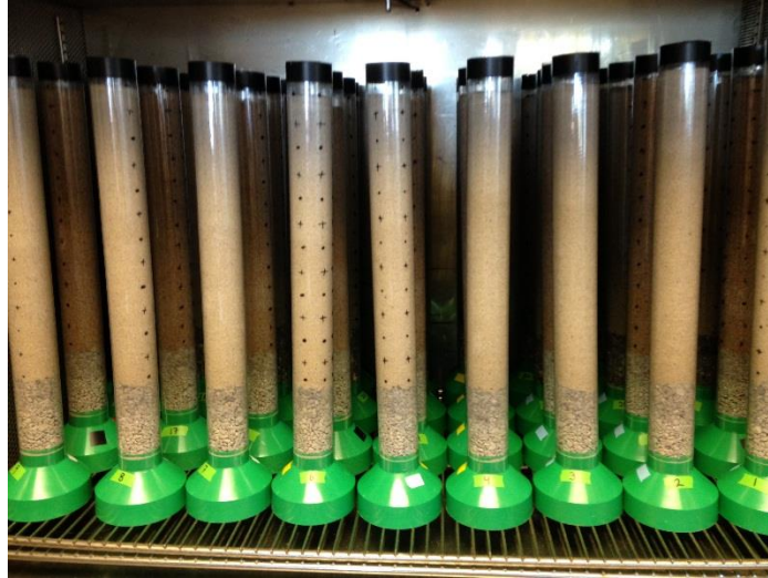
Figure 1. Columns were constructed to meet the recommendations of the USGA for putting green construction.
