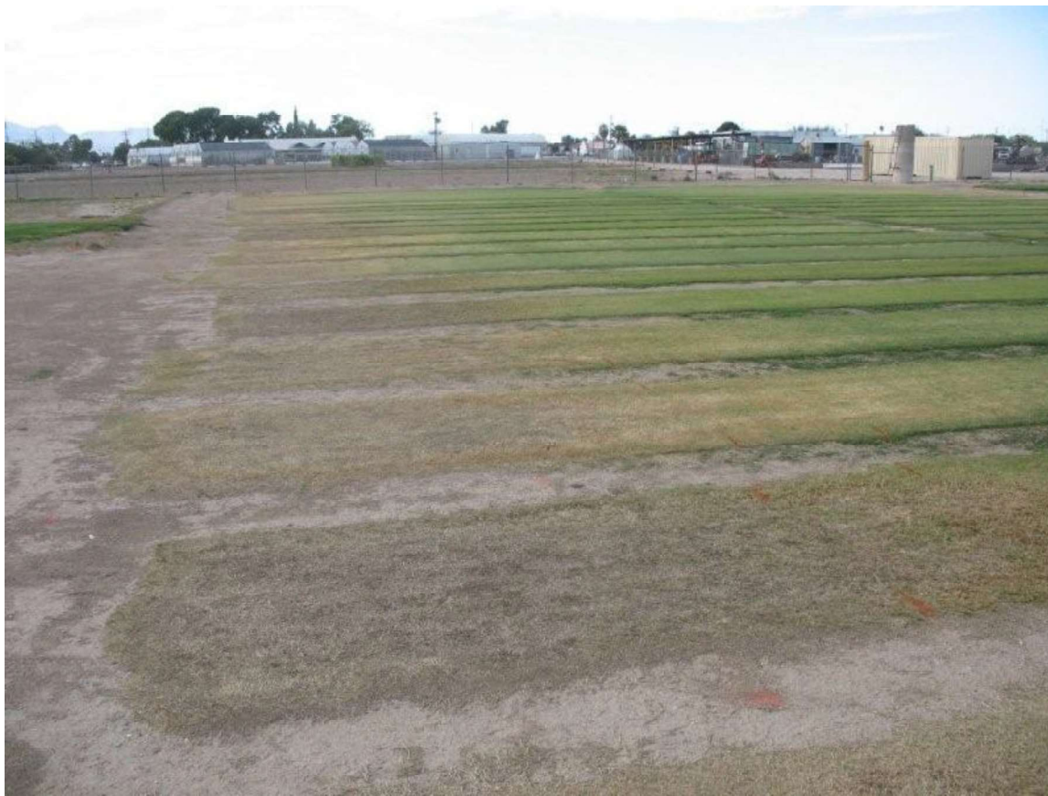
Figure 2. This Linear Irrigation Gradient (or LIGA) design applies a continuous gradient of water from the center sprinkler line that decreases in relative amount with distance to end of the sprinkler radius of throw. The LIGA design here applied irrigation replacement amounts at 75, 65, 55, 45, 35, and 25% of reference ET. Note poorer quality at the ends of plots where irrigation was least.
