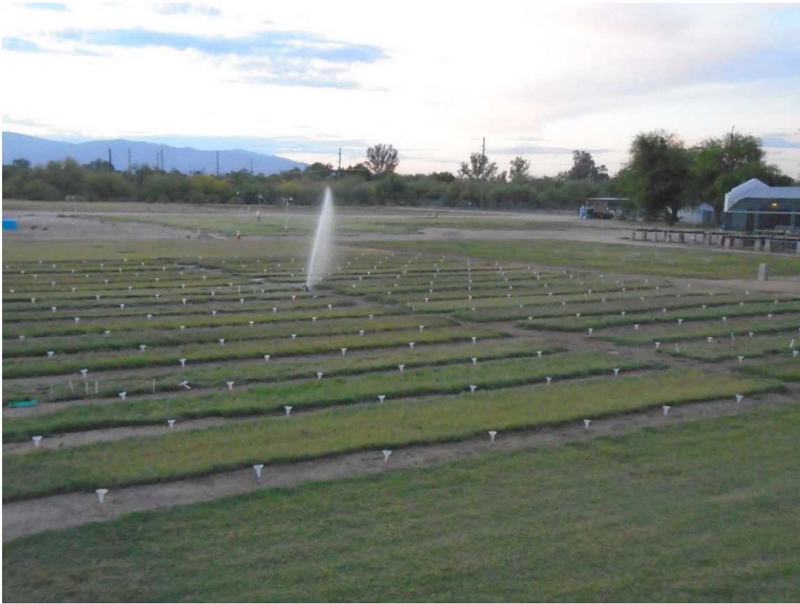
Figure 1. Four cultivars of low maintenance bermudagrass, and three buffalograsses (representing three generations of turf-type development) were tested in 2017 using a special field arrangement referred to as a Linear Irrigation Gradient (or LIGA) design, which was audited to estimate the precipitation rate gradient.
