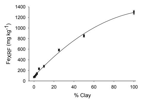
Figure 1. Calibration of an automated XRF stand with soil standards of known clay concentration. Iron is used as a tracer for clay. Each sampling cluster on the graph above actually contains data points from 10 separate scans. This robust method will allow us to track clay movement very accurately.
