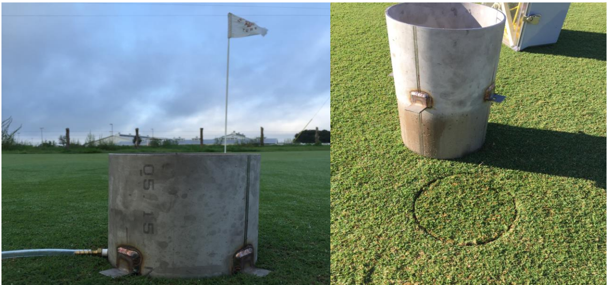
Figure 3. Permeameter to test in situ infiltration rates and near-surface water retention in putting greens.
