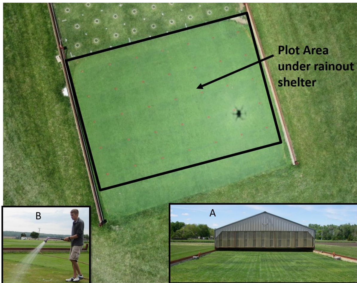
Figure 1. Aerial view of creeping bentgrass plots (top, highlighted with black border). Precipitation was excluded from plots by an automated rainout shelter (inset A), which covered plots during rainfall. This allowed precise irrigation amounts to be applied to individual plots (inset B).
