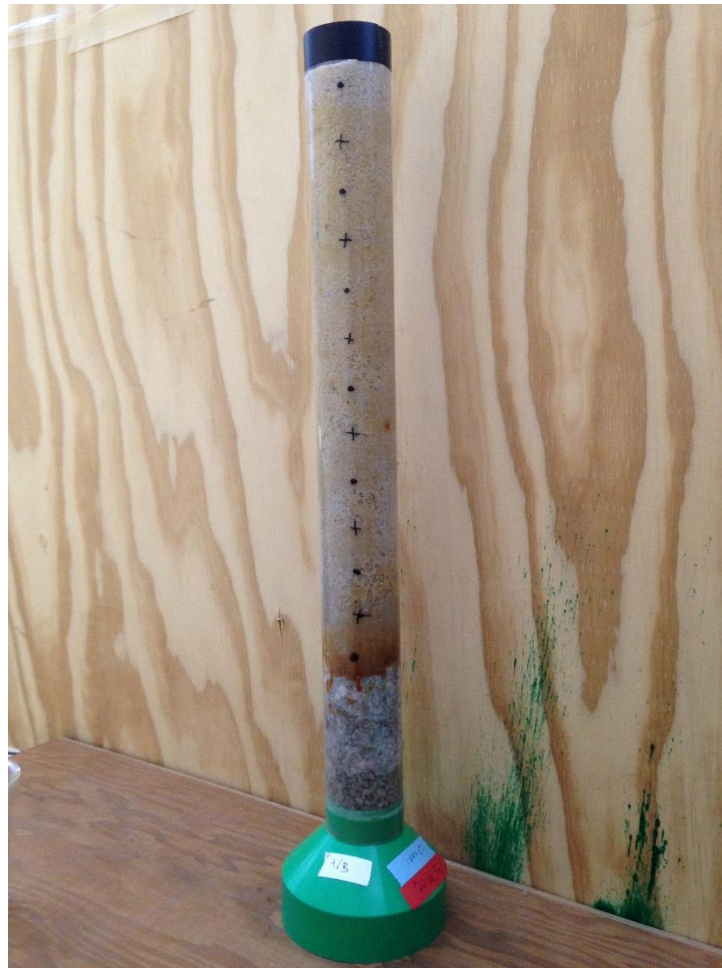
Figure 3. Iron-cemented layer at the sand/gravel interface of a root zone with a low-pH sand and a high-pH gravel. The column received eight total applications of Fe at a rate of 200 \text{ kg FeSO}_4 \text{ ha}^{-1} .
