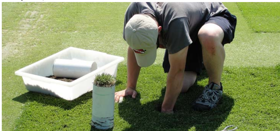
Twenty-four daily ET_a (using weighing lysimeters) and ET_0 (using FAO 56 equation) measurements were used to derive K_c values (calculated as ET_a/ET_0 ) during the summer months beginning June 21 and ending August 31, 2011.
