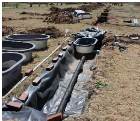
Plastic containers in half the experimental units will be filled with pea gravel instead of slag for use as an experimental control.
