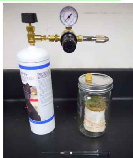
Apparatus for determining the effects of ethylene exposure to creeping bentgrass.
