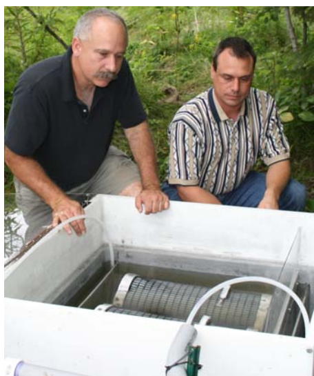
This research is designed to address the potential for end-of-tile filters to significantly reduce the transport of nutrients and pesticides from golf course tile drainage outlets to surface waters.
