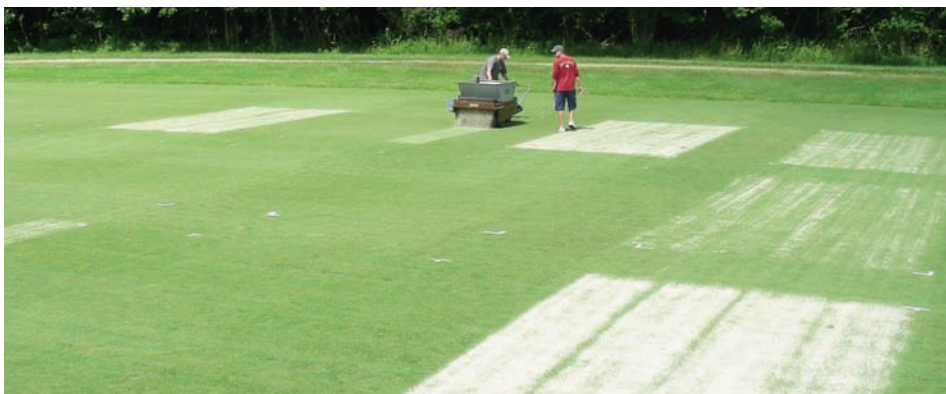
Topdressing applications are kept constant and are applied once per month starting in May and ending in November. This design allows the comparisons of each sand type applied at each of the three rates.
