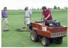
A total of 12 sensors were installed on each fairway to measure temperature, volumetric water content, and electrical conductivity of the soil.
