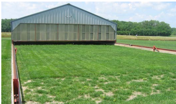
A large rainout shelter at the Rocky Ford Turfgrass Research Plots near Manhattan, KS offers a unique opportunity to compare the irrigation requirements of multiple turfgrass cultivars in the stressful climate of the transition zone.
