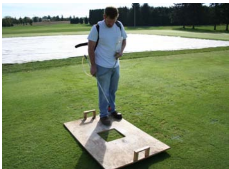
Both urea and ammonium sulfate applications were made to 1 ft 2 plots using a single-boom backpack-type sprayer. Treated plots were covered with a plywood sheet with 1 ft 2 hole cut out of the middle to limit the amount of land treated with 15 N.
