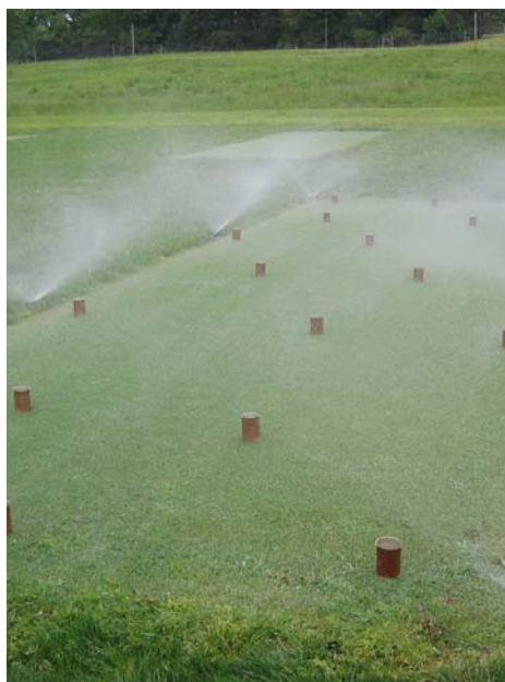
The irrigation system was calibrated with cans to ensure that water was uniformly distributed across each 5 ft x 10 ft subplot.
