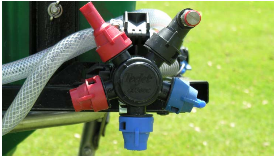
Fungicides were applied using one of five nozzle types designed to distribute varying droplet sizes.
