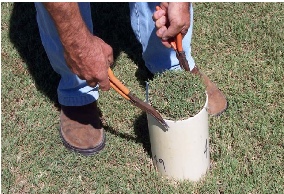
Using weighing lysimeters made from PVC, the consumptive water use rates were determined in 2005 and 2006 for 'Sea Isle 1' seashore paspalum, 'Tifway' bermudagrass, and A48 and A119 inland saltgrass.
