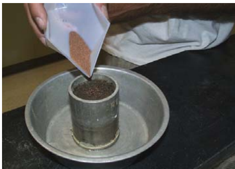
Ash was applied to the surface of the rootzone in the cylinder prior to compaction as well as treatments of applying ash to the surface and worked it into the top 4 mm.
