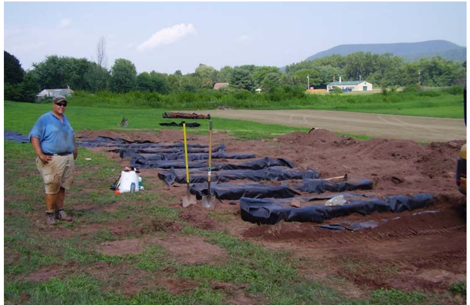
A runoff plot, consisting of 12 vegetative filter strips (4.6m x 0.9m x 1.8m), has been established at the UMASS Turfgrass Research Center, South Deerfield, MA. All plots had a 5% slope and each was lined with impermeable 36-mil polypropylene liners.
