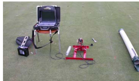
Root growth was monitored biweekly in both studies by using the minirhizotron imaging technique
