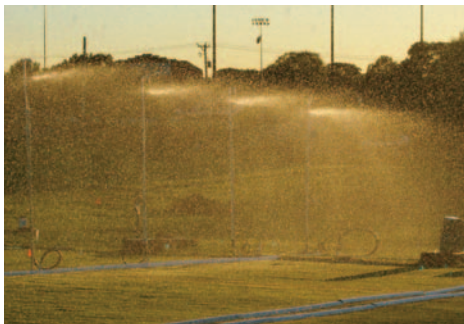
Two rainfall simulations and collection of resulting runoff were conducted to help identify management practices that maximize pesticide and nutrient retention at the site of application.
