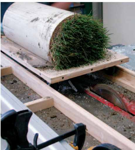
In the fall of 2000, 56 polyvinyl chloride microplots (shown above) were installed in the plot area adjacent to the lysimeters. Microplots were extracted and partitioned into verdure, thatch, roots, and soil on seven sampling dates to evaluate the fate of labeled nitrogen among turfgrass and soil components.
