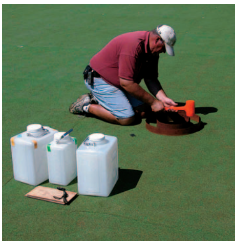
Field water infiltration rates were considerably lower than what might be anticipated based on K_{sat} values, and sand size had a significant effect on infiltration with coarser sand mixes having higher infiltration rate than finer sand mixes.
