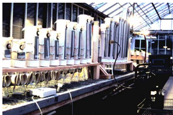
Research is underway to quantify water content and movement in various putting green rootzone mixes and to document how depth of the rootzone and profile construction can affect those parameters.
