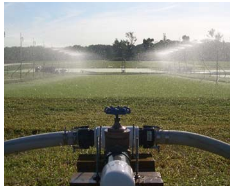
A rainfall simulator is being used to generate runoff events for this experiment.
