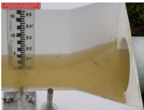
Trapezoidal flume and line from a bubble flow meter used to monitor discharge from a runoff event
