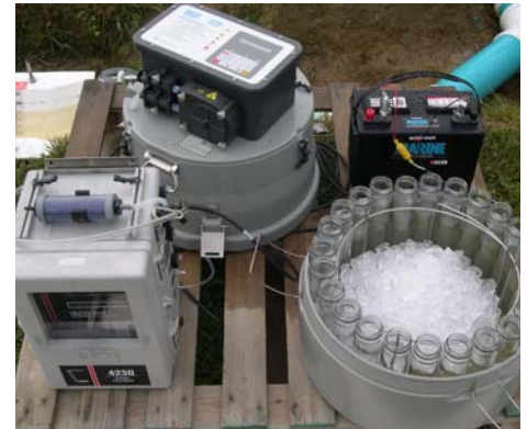
Bottles are pre-cooled with ice prior to sample collection to minimize chemical transformations that may occur prior to transport to the laboratory.
