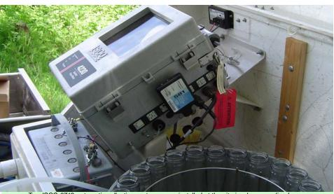
Two ISCO 6712 automatic collection systems were installed at the site in when sampling began.
