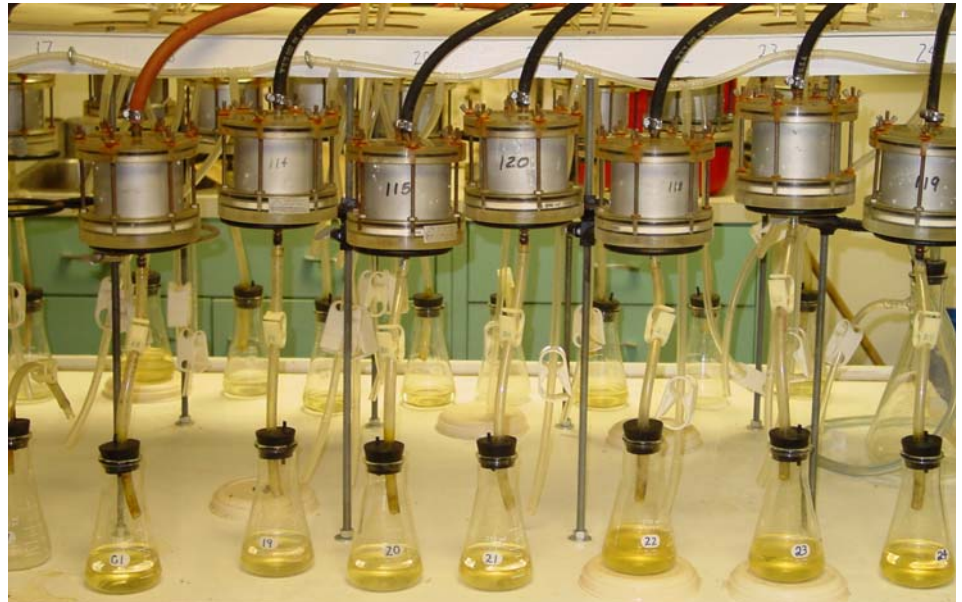
In the lab, this apparatus is used to measure the infiltration rate of cores collected in the field.
