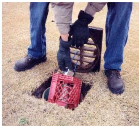
A special type of glass bottle that sealed automatically after filling with runoff was used to detect pesticides.
