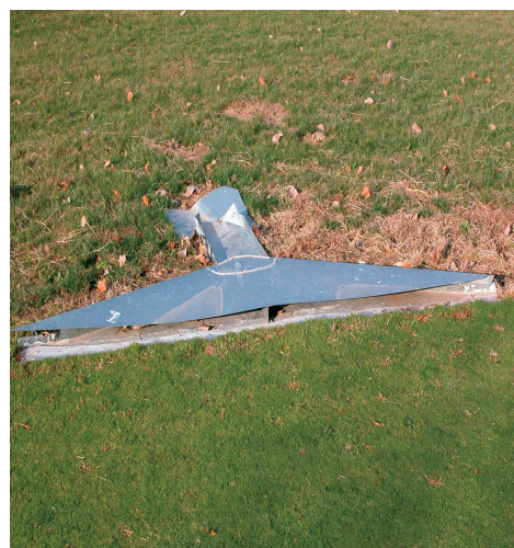
At the base of each plot is a collection flume that funnels the runoff into a small pit.
