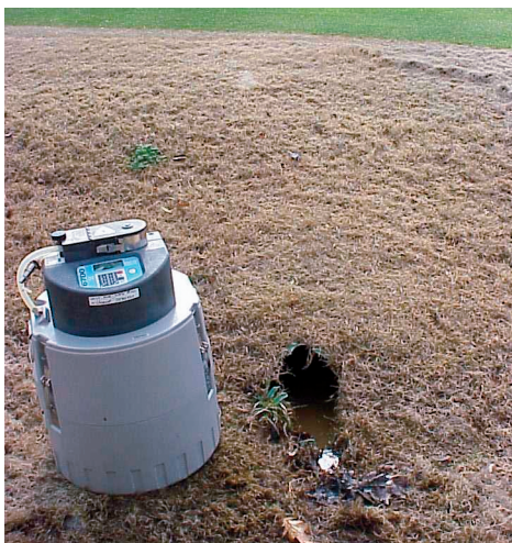
Automatic samplers are used to collect fairway runoff water during rainstorm events.
