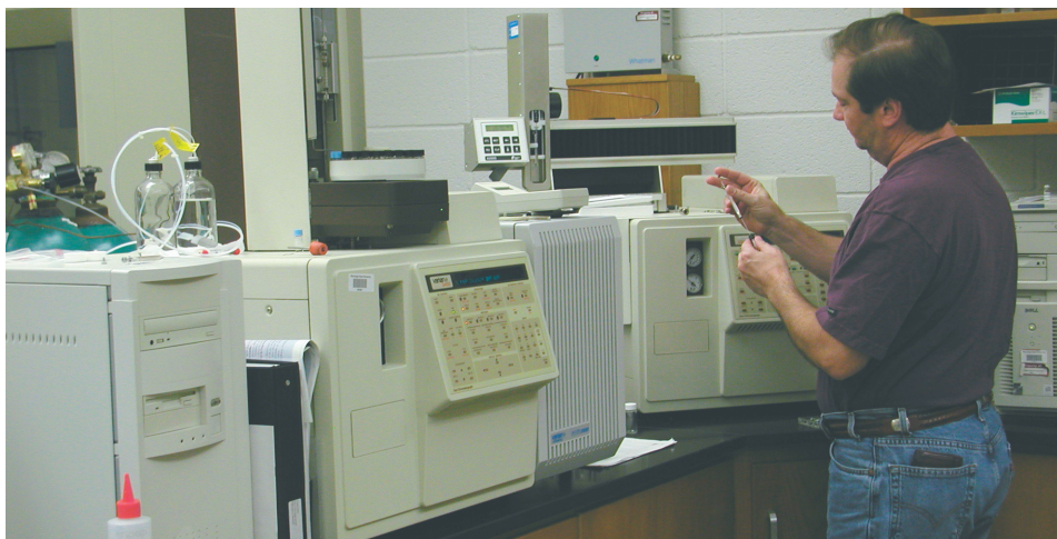
Analytical methods developed to detect pesticides included both gas and liquid chromatography.
