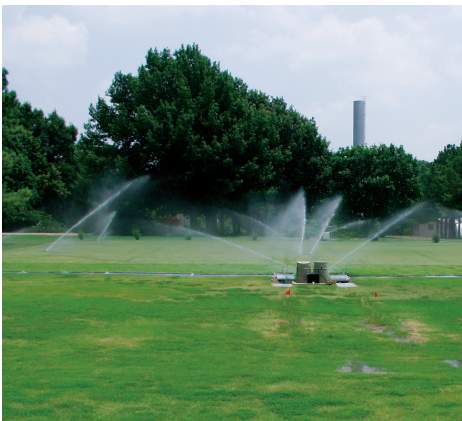
Runoff is collected from both natural and simulated rainfall. The irrigation system produces simulated events up to two inches per hour with an 80% coefficient of uniformity.
