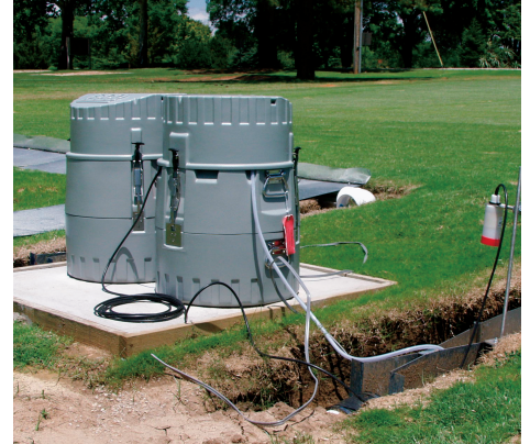
Automatic samplers record flow rate and collect runoff at user-determined intervals after an ultrasonic detector sense the presence of runoff.
