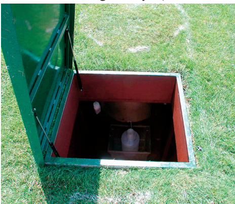
Lysimeter where leachate samples are collected for long-term N fate research.
