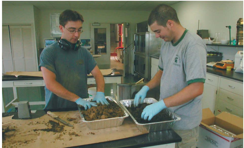
Separating soil from microplots for 15 N analysis
