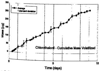
A volatilization flux chamber (16 in. X 16 in.) was placed directly on the turf in each designated plot. The air above the turfgrass surface was pulled out of the chamber at a very low rate (approximately 10 liters/minute). The cumulative mass of chlorothalonil that volatilized from the putting green plots was 0.017% of the total applied mass.
