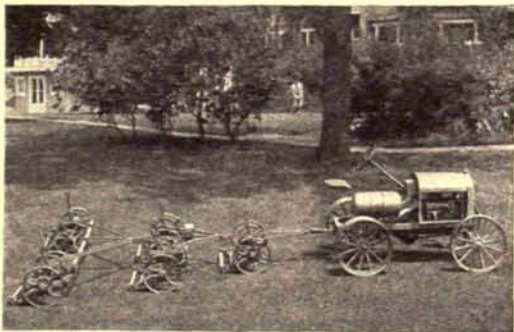
Tractor and five-unit gang of fairway mowers manufactured and shown by the Worthington Mower Company, Stroudsburg, Pa.
