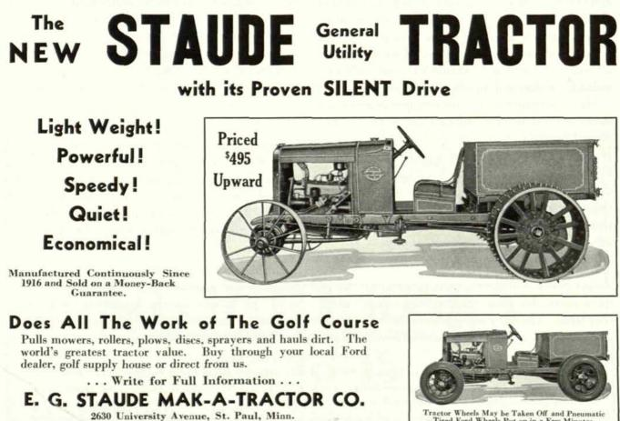
Tractor Wheels May be Taken Off and Pneumatic Tired Ford Wheels Put on in a Few Minutes.
