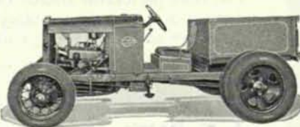
Steel tractor wheels demountable. May be replaced by Ford pneumatic tired wheels for paved roads.
